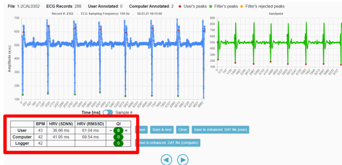
Figure 5.5: The three BPM values (user, logger, and computer) can be seen in the red box on the bottom left.
