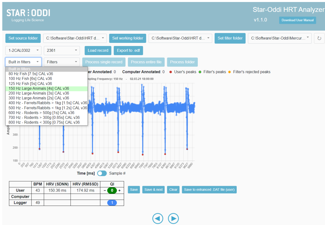
Figure 5.3: The list of available sampling frequencies using the the built in filters. The recommended filter is highlighted in green.
